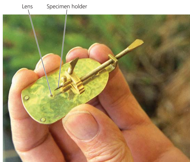
▲ FIGURE 1.2 Reproduction of Leeuwenhoek's microscope. This simple device is little more than a magnifying glass with screws for manipulating the specimen, yet with it, Leeuwenhoek changed the way we see our world. The lens, which is convex on both sides, is about the size of a pinhead. The object to be viewed was mounted either directly on the specimen holder or inside a small glass tube, which was then mounted on the specimen holder.
